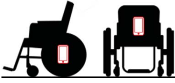
Figure 1. Location of the smartphone on the wheel (left); Location of the smartphone at the back of the seat (right)
